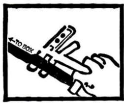
With your left thumb pressed tightly over the strap on the corner of the carton, facing you, securely grip the tension tool and pull toward yourself until desired tension is achieved.
