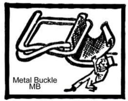
Loop end of strap and insert through Buckle as shown, Loop over open end of wire.
