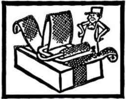
Encircle package, bundle or pallet with strap - make a loop and insert through buckle over end of wire as shown in Illustration.
