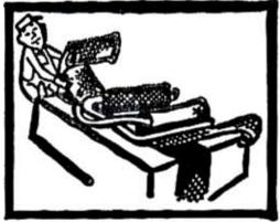
After slipping loop over end of buckle, hold package securely and tension strap around package using 31 Hand Pull (See directions below).
