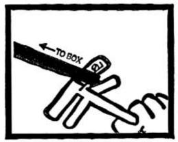
Disengage tool from strapping by reversing the previous operation. Insert the excess strapping between cutting and safety bars. Cut off the strap approximately 2 to 4 inches away from the metal buckle.
