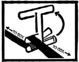
Rotate tool 180° counterclockwise upward with right hand and then downward toward metal buckle, keeping strap tight on tool as shown to avoid slipping
