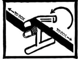
Complete the 360° counterclockwise rotation as shown. Keep proper strap alignment in order to achieve maximum tension when pulled.
