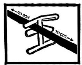
Excess strap from coil should be pulled and held tight by left hand. Hold tension tool in right hand. Insert excess strapping between the pulling and locking bars as shown.
