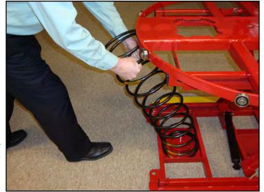
7. Grasp the spring by the second or third coil down from the top (do <u>NOT</u> grasp the top coil or rung) and push the spring down and under the edge of the top frame.
