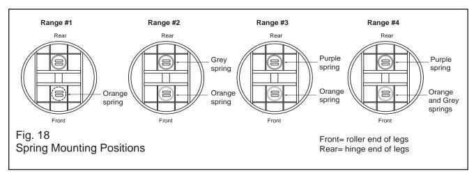
13. Figure 4 shows the position of additional springs if needed. Double-check to be sure you have the correct springs. Refer to Table 1 on page 10 and see that you have the correct springs for your application.
