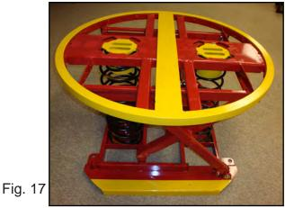
12. Reinstall the rotator ring.
