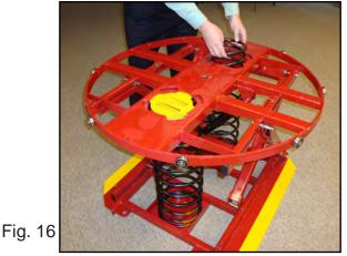
11. Install additional springs as needed through the bayonet openings. Reinsert the yellow bayonets and twist to lock them in place.
