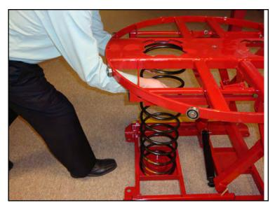
8. While pushing down to compress spring push it forward into the pocket up under the top frame. It will "snap" into position when completely in the pocket.
