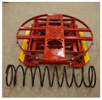
2. The unit is shipped without springs installed. The installation of the first spring (orange) requires two people. Lift off rotating ring and both yellow bayonets. Set them aside, they will be installed later.
