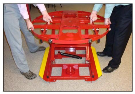
4. With the help of an assistant, lift the top frame until it hits the upper latch stops.
