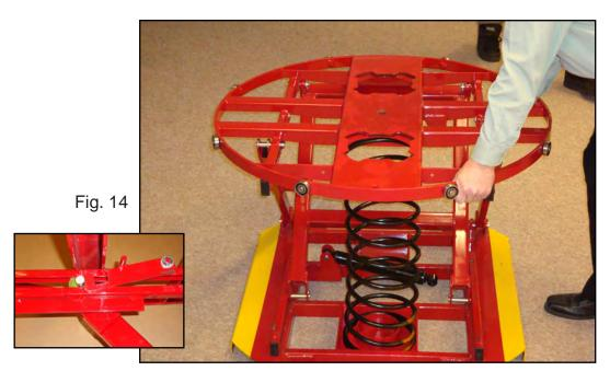
Remove the shock absorber pivot pin. Push down on top frame until latches engage. (Both latches will drop into place).
