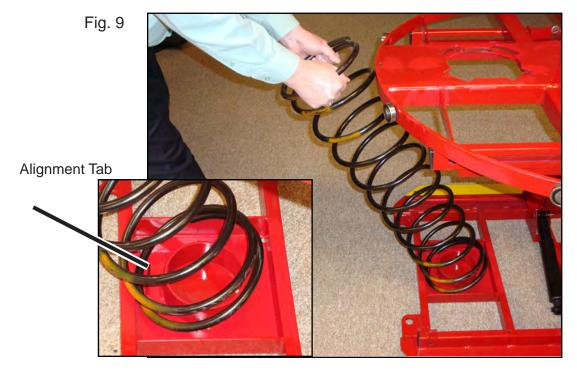
Insert either end of the large orange spring into the lower pocket. Be sure the bottom spring coil is positioned outside the alignment tab as shown.
