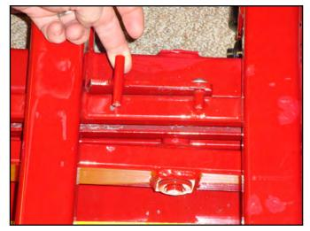
While holding both latches up and lift the top frame pass the latches until it is at its full, upper most position. Have the assistant hold the weight and insert the pivot pin in the hole in the base frame. See Fig. 8. With the PalletPal in this full upper most position the orange spring can be installed.
