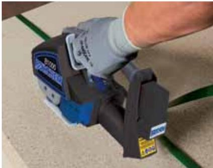
The B1000 can pull up to 1125lbs of tension and operate with both polypropylene and polyester plastic strapping, 5/8" to 3/4" wide, .031-.050" thick. No special change parts are required to adjust for strap width or thickness. The 14.8V Lithium Polymer (LiPo) battery weighs less and is more efficient in power output compared to Nickel-Cadmium and Lithium Ion batteries of higher voltage. Plus it can be fully re-charged at ANYTIME without memory loss.
