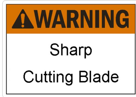
The label shown is affixed to the upper tape head assembly on either side of the machine. It warns operators and service personnel of the presence of the cutting blade that may not be visible. Caution should be exercised when approaching this area
