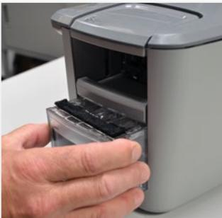
Eject and fill the water tank, then insert it back into place.
