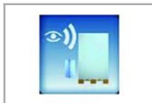
Icon **(D1)**: used to select the automatic stop of the spool carriage (lifting phase) depending on the height of the pallet being wrapped.
