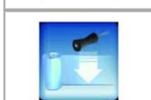
**(O)** Push-button: used to enable and disable the programming of the cycle with creasing device (Optional). If the electric creasing device is available, you can set the folding percentage.
