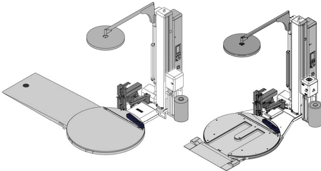
**Rotating platform machine for plastic stretch film wrapping**
