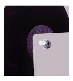
B. Unwind Felt Slip Disk: This braking surface should be periodically checked to ensure that the felt disk is clean and dry. If this disk has excessive dirt or oil, replace with part #75806.
