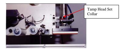
9. Set the tamp stroke by placing the product under the tamp pad. Disconnect the air supply and move the tamp pad to the product to be labeled. Loosen the tamp head set collar so it limits the stroke of the tamp head, tighten collar and reconnect air supply.
