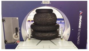
Gravity rollers embedded on infeed and outfeed tables provide a smooth transition into the wrap zone while helping direct the product into the center of the guide rollers.
