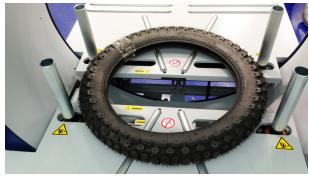
Self-centering guides center product in the ring and automatically rotate the product to provide a smooth, contiguous wrap--suitable for shipping.
