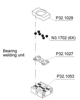
All other parts have to be greased due to the explosion drawing. Lubrication interval: While each maintenance
