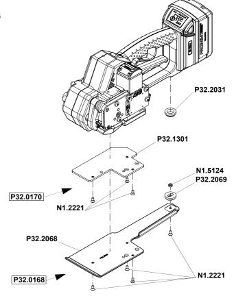
If the complete bottom side of the tool has to be protected, the plate P32.0168 must be used.
