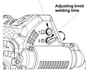
The adjustment knobs can be easily turned with a coin.
