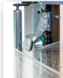
Film roping, with chain drive
